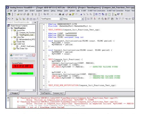
Figure 1: Screen capture of the *Embedded-Unit* tests for initializing the Blackfin core timer via two apparently equivalent C++ routines (Lines 11 – 12 and 16 -- 17). Undocumented silicon level behaviour resulted in one assert unexpectedly failing (Line 29), and another unexpectedly passing (Line 30). (From [Smith et al, 2009a]).
